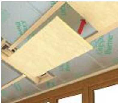
Install insulation between batten
